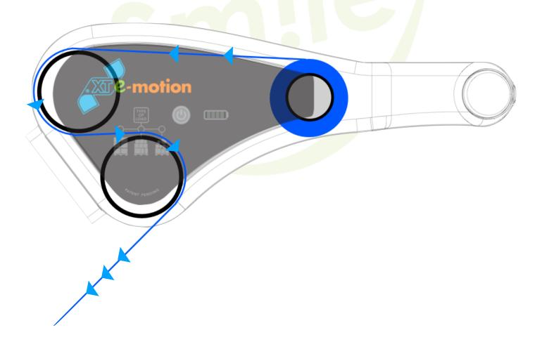
The XTE-motion® dispenser has a quick load system for the roll of Strigta® film.
